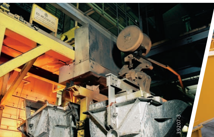
DH hoist in a foundry for safely handling molten masses Full-portal crane with DH hoist units in tandem mode
