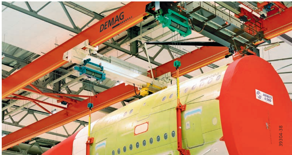
4 synchronised DH hoists for precise transport of aircraft fuselage segments
