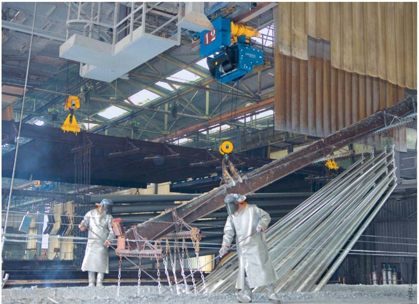
Demag FDR foot hoists travelling on a semi-automatic circuit in a galvanizing plant.
